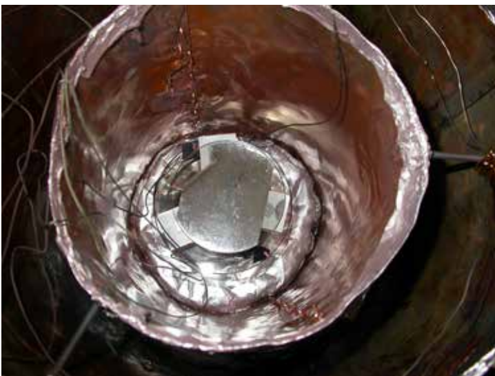
Figure 3, Specimen group installed in a vertical interferometer.
